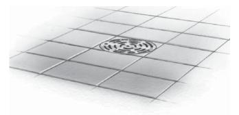
8. Infill or lay floor screed and apply final floor finish (e.g. tiles, marble, paviors, terrazzo) around the grating or cover.
