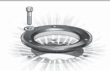
6. Where applicable, dress the membrane over the flange and into the sump of the body, ensuring that the membrane does not restrict the outlet; bolt the membrane clamping collar to the body – certain collars are reversible to increase height adjustability.
