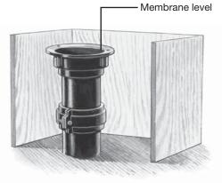
Connect body (with spigot adaptor if applicable) to pipework.
