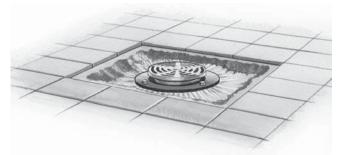
7. Fit grating, cover, or funnel with extensions, frame or collar as applicable; set top face flush and level with the finished floor using height adjustability features. Use a suitable, good quality sealant on all threaded joints to ensure a watertight assembly.
