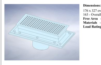
176 x 327 overall size 163 - Overall Height Free Area - 95cm<sup>2</sup> Materials - Stainless steel Load Rating Class - K3
