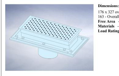
176 x 327 overall size 163 - Overall Height Free Area - 100cm<sup>2</sup> Materials - Stainless steel Load Rating Class - K3
