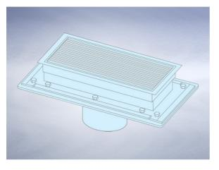
Dimensions: 176 x 327 overall size 163 - Overall Height Free Area - 245cm<sup>2</sup> Materials - Stainless steel Load Rating Class - L15
