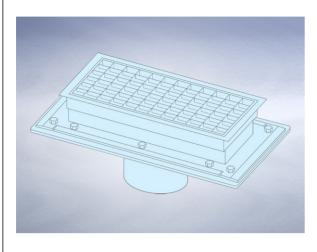
176 x 327 overall size 163 - Overall Height Free Area - 360cm<sup>2</sup> Materials - Stainless steel Load Rating Class - L15
