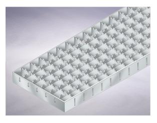
200 x 500 overall size 23 - grating aperture width 30 - Depth Free Area - 1620 per metre Materials - Stainless steel Load Rating Class - B125 Weight - 2.3 kg
