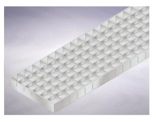
300 x 500 overall size 23 - grating aperture width 40 - Depth Free Area - 2440 per metre Materials - Stainless steel Load Rating Class - B125 Weight - 2.3 kg
