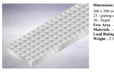
200 x 500 overall size 23 - grating aperture width 30 - Depth Free Area - 1620 per metre Materials - Stainless steel Load Rating Class - B125 Weight - 2.3 kg
