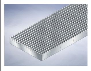
150 x 1000 overall size 5 - grating aperture width 20 - Depth Free Area - 825 per metre Materials - Stainless steel Load Rating Class - A15 Weight - 3.4 kg
