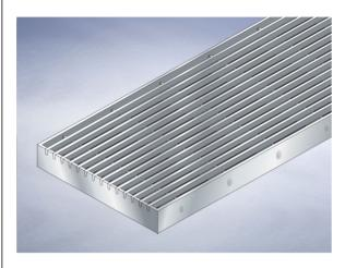
135 x 500 overall size 5 - grating aperture width 20 - Depth Free Area - 740 per metre Materials - Stainless steel Load Rating Class - A15 Weight - 1.5 kg
