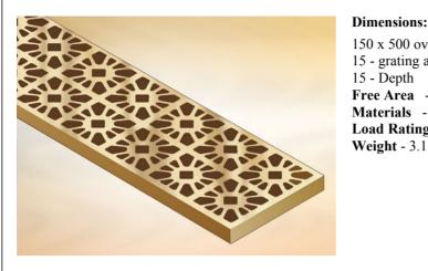
150 x 500 overall size 15 - grating aperture width 15 - Depth Free Area - 475 per metre Materials - Nickel bronze Load Rating Class - A15 Weight - 3.1 kg
