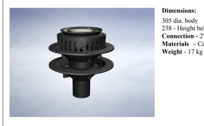
305 dia. body 238 - Height below Body Flange Connection - 2" BS416 / Harmer SML Materials - Cast iron, lacquered
