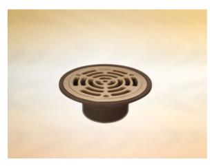
Dimensions: 129 dia. at finish level 142 dia. overall size 54 - Overall Height Connection - 82mm Plastic, 75mm DIN19522 / Harmer SML Free Area - 32cm<sup>2</sup> Materials - Grating - nickel bronze; Frame - cast iron, sherardized Load Rating Class - L15 Weight - 1.1 kg
