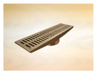
Dimensions: 125 x 430 at finish level 70 - Overall Height Connection - 110mm Plastic, 100mm DIN19522 / 4" BS416 / Harmer SML Free Area - 155cm<sup>2</sup> Materials - Nickel bronze Load Rating Class - L15 Weight - 5.6 kg
