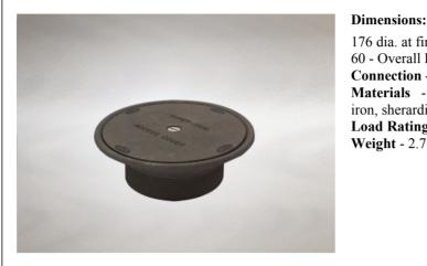
176 dia. at finish level 60 - Overall Height **Connection - 4**" NPSM Vari-Level thread **Materials** - Cover - ductile iron, sherardized; Frame - cast iron, sherardized **Load Rating Class -** M125 **Weight -** 2.7 kg
