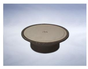
Dimensions: 160 dia. at finish level 176 dia. overall size 60 - Overall Height Connection - 110mm Plastic, 100mm DIN19522 / 4" BS416 / Harmer SML Materials - Cover - stainless steel; Frame - cast iron, sherardized Load Rating Class - L15 Weight - 2.4 kg
