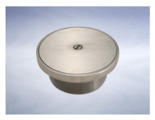
Dimensions: 150 dia. at finish level 53 - Overall Height Connection - 110mm Plastic, 100mm DIN19522 / 4" BS416 / Harmer SML Materials - Stainless steel Load Rating Class - L15 Weight - 1.4 kg
