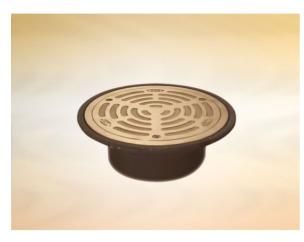
Dimensions: 160 dia. at finish level 176 dia. overall size 60 - Overall Height Connection - 110mm Plastic, 100mm DIN19522 / 4" BS416 / Harmer SML Materials - Cover - nickel bronze; Frame - cast iron, sherardized Load Rating Class - L15 Weight - 2.5 kg
