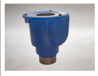
Dimensions: 265 dia. body 304 - Height below Body Flange -30 to 10 - add to overall grating/cover height for min/max height between body flange and FFL Connection - 4" BS437 (100mm) / Harmer SML Free Area - 78cm<sup>2</sup> Materials - Cast iron, lacquered Weight - 17.3 kg Note: Membrane clamping collar C.D also required if using with a Vari-Level top (C.M1 with Multi-Level). (priced separately from body)
