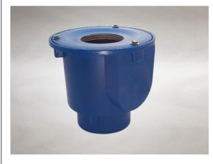
Dimensions: 265 dia. body 240 - Height below Body Flange -30 to 10 - add to overall grating/cover height for min/max height between body flange and FFL Connection - female 4" BSP threaded connection (100mm) Free Area - 78cm<sup>2</sup> Materials - Cast iron, lacquered Weight - 11.6 kg Note: Membrane clamping collar C.D also required if using with a Vari-Level top (C.M1 with Multi-Level). (priced separately from body)
