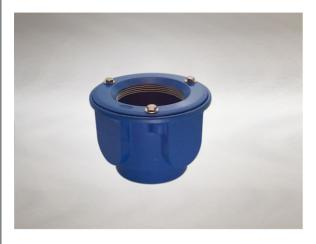
Dimensions: 200 dia. body 135 - Height below Body Flange -30 to 10 - add to overall grating/cover height for min/max height between body flange and FFL Connection - female 2" BSP threaded connection (50mm) Free Area - 19cm<sup>2</sup> Materials - Cast iron, lacquered Weight - 7.6 kg Note: Membrane clamping collar C.C3 or C.C also required if using with a Vari-Level top. (priced separately from body)
