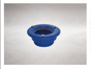
Dimensions: 200 dia. body 75 - Height below Body Flange -30 to 10 - add to overall grating/cover height for min/max height between body flange and FFL Connection - female 2" BSP threaded connection (50mm) Free Area - 19cm<sup>2</sup> Materials - Cast iron, lacquered Weight - 2.8 kg Note: Membrane clamping collar C.C3 or C.C also required if using with a Vari-Level top. (priced separately from body)
