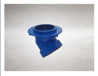
Dimensions: 188 dia. body 162 - Height below Body Flange -15 to 5 - add to overall grating/cover height for min/max height between body flange and FFL 162 - depth body flange to outlet center line Connection - female 4" BSP threaded connection (100mm) Free Area - 78cm<sup>2</sup> Materials - Cast iron, lacquered Weight - 3.5 kg
